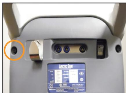
Fig. 8-72 Retire el perno (paso 1)
