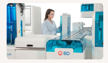
BD® Kiestra Total Laboratory Automation System (third generation), a fully automated robotic track system for microbiology labs that connects different Kiestra modules in a flexible and customizable way and automates lab specimen processing.
