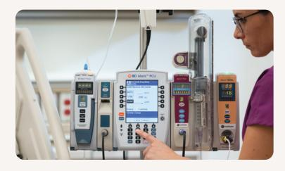
**BD® Alaris® Infusion System,** a modular and comprehensive infusion system that includes large volume pumps, syringe pumps, patient-controlled analgesia (PCA) pumps, respiratory monitoring, dose error reduction software and electronic medical record (EMR) interoperability.
